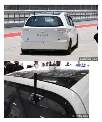
Not much has changed with the exterior since then, with additional LED light strips and prominent MyKar badging at the rear of the car – along with two signal antennas on the upper section of the rear lid – being the most visible changes.
